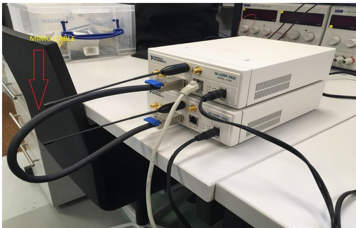
Figure 6. Transceiver USRP set-up.
